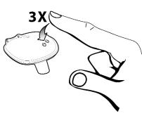
Your finger should be moist, but not dripping, before you touch the Wet Switch $^{\text{TM}}$ . You can achieve the correct dampness by dipping your finger in water, then dabbing your finger twice on a towel.
