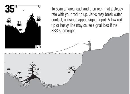
The returned "echoes" are transmitted with wireless technology to the display unit and plotted on the LCD. New information appears on the right. As this information moves to the left a very accurate picture of the underwater world is created, including the depth of underwater objects such as the bottom, fish, and structures.
